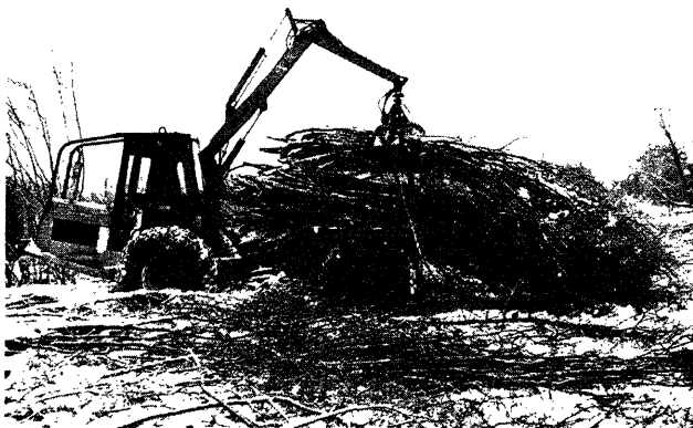
Figure 3.--Forwarding bunched alder to roadside.
