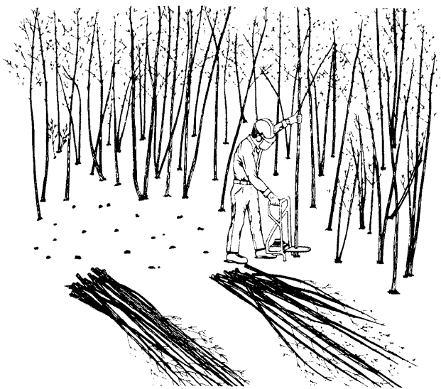
Figure 2.--Illustration of felling and accumulating small trees with the Finnish felling frame.
