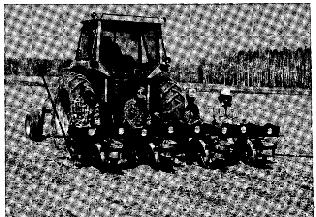
Figure 6.—A four-row mechanical transplanter can plant unrooted hardwood cuttings at a rate of 5,000/hour at a 3.3 x 3.3 ft spacing.
