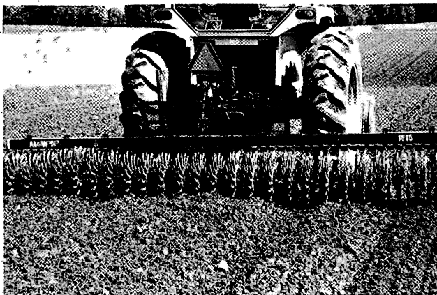
Figure 9.—A rotary hoe controls weeds both between and within rows but can be used only during the first 6 weeks when the trees are less than 1 foot high.
