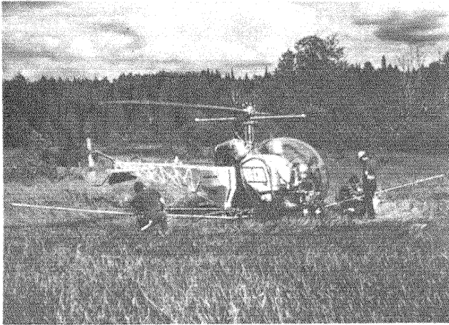
Bell 47 helicopter being made ready for liftoff; it is equipped with two Beecomist 350 rotary spray nozzles with 100-micron sleeves.
