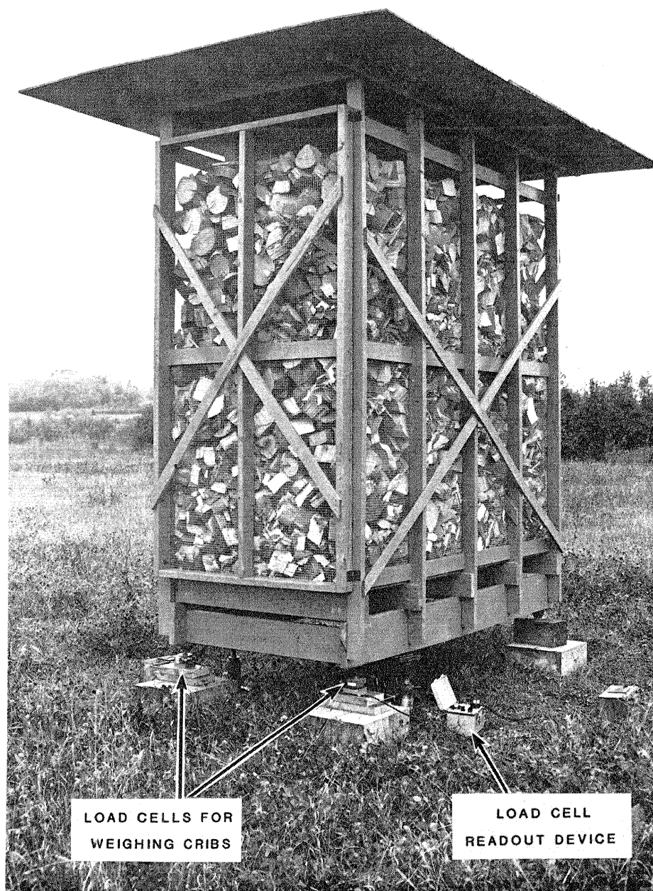
Figure 6.—Test setup for outdoor crib air drying experiment.
