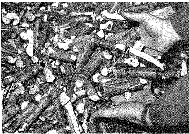
Figure 9.—Billets produced from chunking bundled stems with the involuted single-disc wood chunker.
