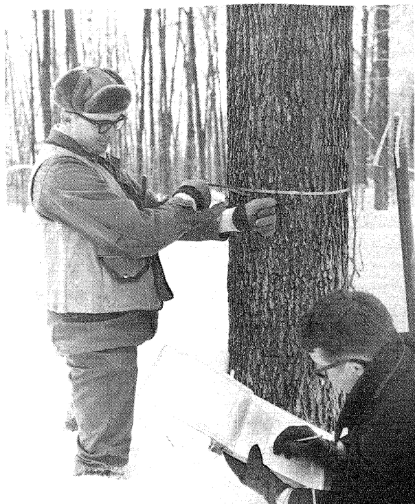
Figure 9. — A field man measures the diameter at breast height (d.b.h.) of a sawtimber-sized tree while his companion records information on plot sheet. Such measurements made on the same trees during the 1956 and 1968 surveys on permanent sample plots provided a value of radial growth accrued between surveys. This information was used to estimate the total volume of growth in the State. (Photo courtesy of Wisconsin Department of Natural Resources.)
