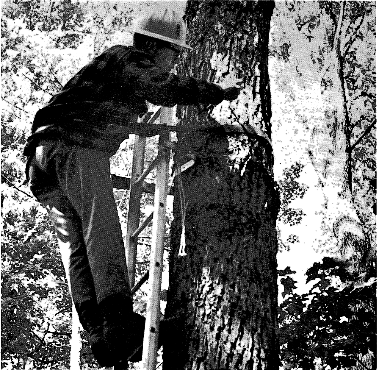
Figure 1.—Collection of field test data. Bark thickness was obtained at various tree heights by using a Swedish bark gauge.
