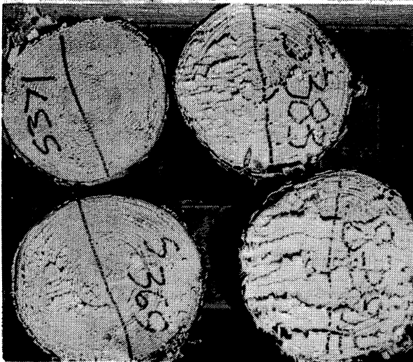
Figure 21. — Cut faces of unfrozen roundwood bolts sheared with dull shear blades (anvil E, 1.5-inch gap).
