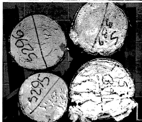
Figure 21. — Cut faces of unfrozen roundwood bolts sheared with dull shear blades (anvil E, 1.5-inch gap).
