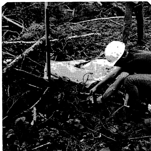
Figure 3. Sheet metal or plastic go-no-go gage may be used to determine fine fuel diameter classes.
