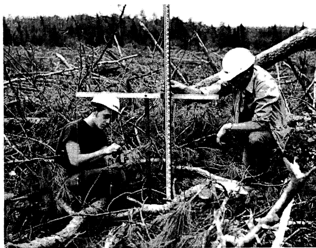
Figure 1. Branchwood particles intersected by the sample line are tallied by species and diameter class. In this photograph the sample is only one meter long, and is delineated in 25 centimeter segments by plumb-bobs suspended from a meterstick. A large number of these short samples must be taken to ensure reliable results.
