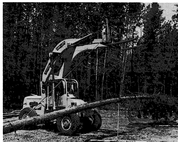
Figure 4.--Setup showing the procedure used in measuring the period of oscillation of the full tree.
