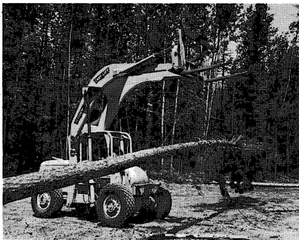
Figure 3.--Setup showing the procedure used in weighing and locating the center of gravity of full trees
