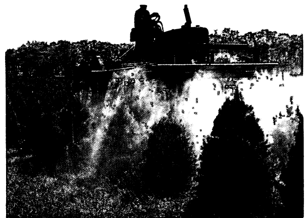
Figure 5.--Hydraulic sprayers such as this straddle type are very effective for applying fungicides to control foliage diseases in Christmas tree plantations.
