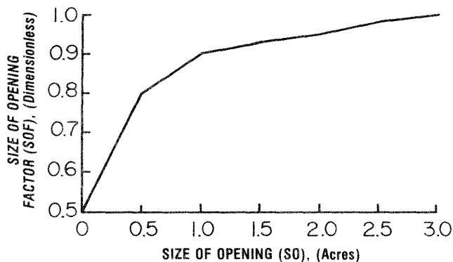
Figure 20.--The small-opening factor, SOF, adjusts timber volumes for losses when opening size is less than 3 acres.
