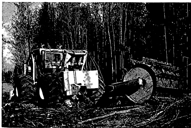
Figure 1.—Pettibone Master 1500 skidder and Fleco Corporation Model SS812 single drum roller chopper.
