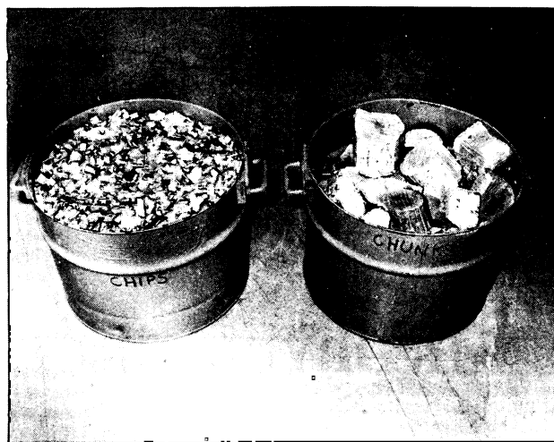
Figure 1.—Test setup for natural convective drying of chips (left) and chunks (right).
