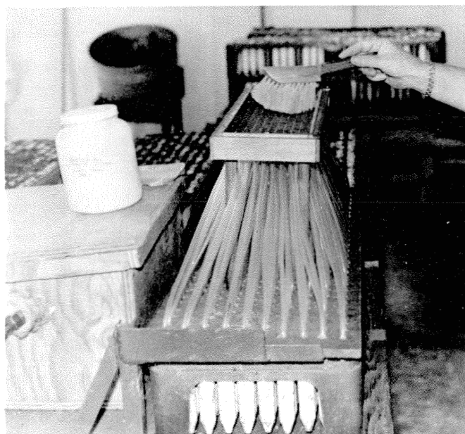
Sowing pelleted seeds into Leach Cone-tainers with a gravity seeder.
