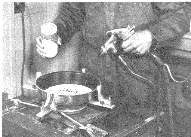
Pelleting seeds with fine sand and a polyvinyl alcohol in a reciprocating-rotating pan.
