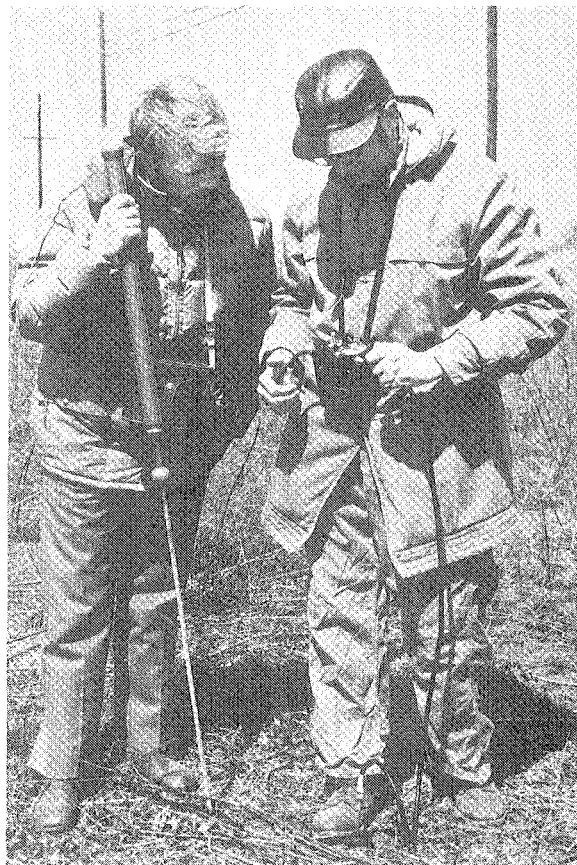
Figure 4.—Bar hole maker is held by man on left. Right, reading an MSA Explosimeter to measure the concentration of combustible gases in a sample drawn from the bar hole.
