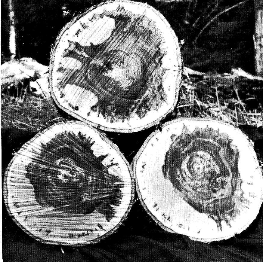
Figure 5. — A jagged pattern of defect associated with a medium infestation. The injured annual ring is distinct in the lower samples. Small dots of discoloration in the upper sample indicate a light recent infestation.
