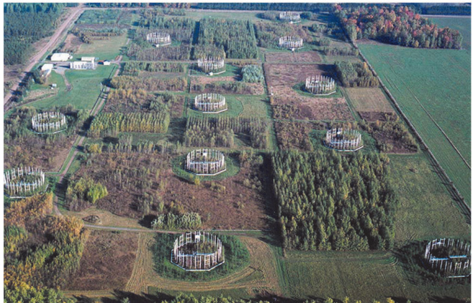
Figure 8.—An aerial view of the FACE study site near Rhinelander, Wisconsin. Each ring consists of 32 vertical vent pipes for emitting CO_2 and O_3 into the growing space for the experimental plant materials.
