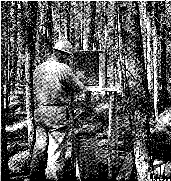
Figure 1. Recording well to measure bog water table fluctuations (left) and stream gauge for measuring run-off from an experimental peat deposit and surrounding catchment (right). (F-498745, F-507718).
