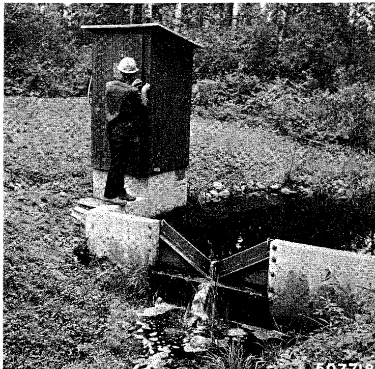
Figure 1. Recording well to measure bog water table fluctuations (left) and stream gauge for measuring run-off from an experimental peat deposit and surrounding catchment (right). (F-498745, F-507718).
