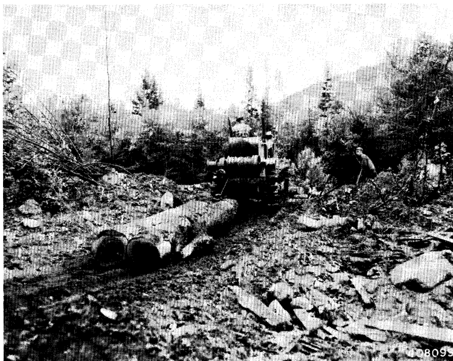
Figure 1.--A 25-horsepower tractor can ground-skid only about 1 ton on an uphill slope.
