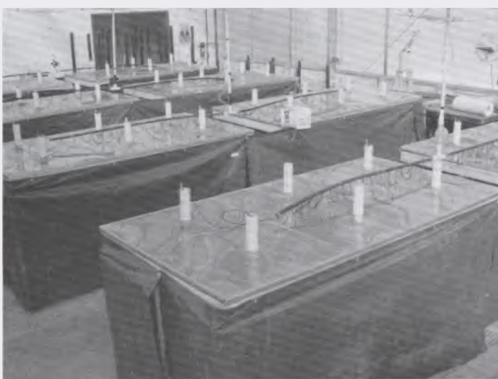
Figure 1. Operational rhizotrons used for two-dimensional, horizontal root growth measurements. Observations of the root systems are taken on the underside of the rhizotrons by removing the tarps.
