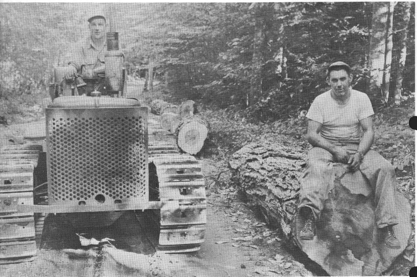
Figure 8.--The old-growth woodlot was logged by a 2-man crew using power saws and a T-6 tractor.
