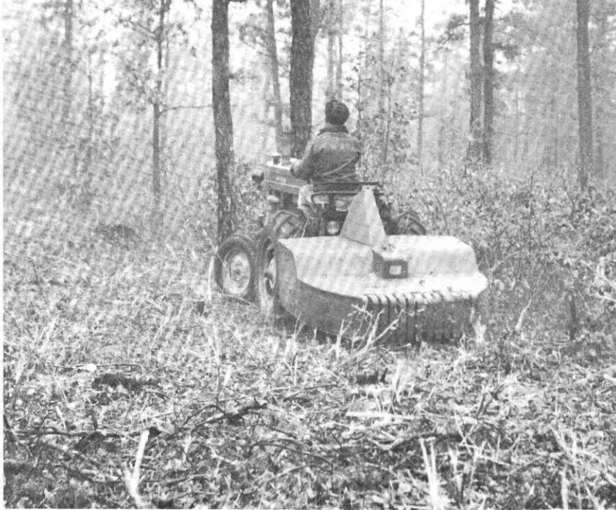
Figure 2.--Brush-hogging one of the scrub oak areas where broadcast sowing of pitch pine seed was tried. The brush hog is like an oversize rotary lawnmower. This one had a 5-foot blade powered by a farm tractor. It easily handled clumps of scrub oaks 4 to 7 feet tall. Usually it severed them about 6 inches above the ground; but in this area, because of stumps, the blade was set a bit higher.
