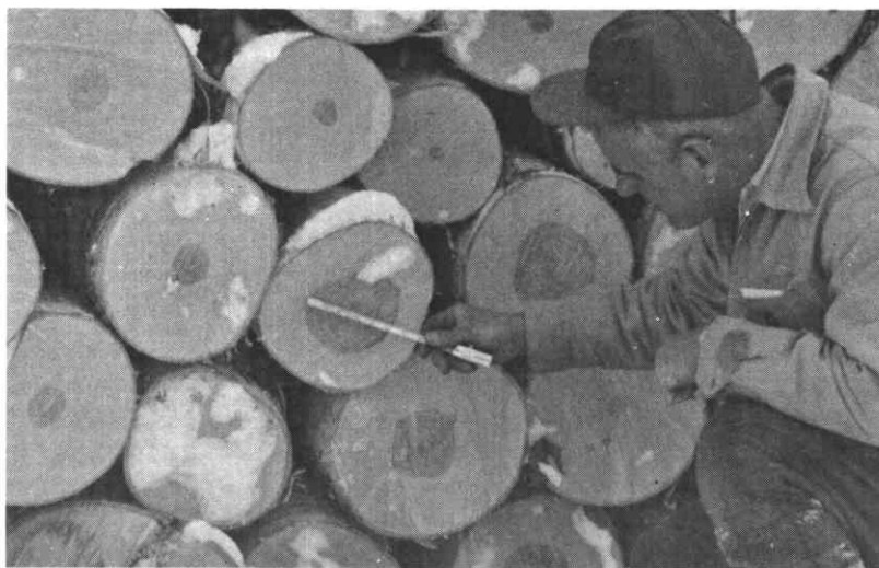
Figure 8.--Red heart is a serious defect in paper birch. A discoloration that resembles heartwood, it is believed to be caused by parasitic organisms.
