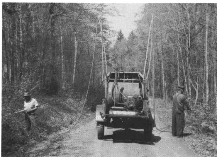
Figure 2.--A power sprayer, converted from a standard-model fire-control pumper, in use on a road on the Monongahela National Forest. The poles hold surplus hose off the ground and out of the way when spraying close to the truck, as shown here. When the full length of the hose is needed, it is easily available.
