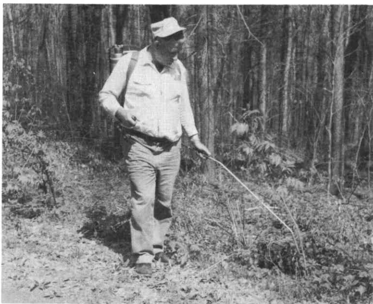
Figure 3.--A. Back-pack sprayer of the type used in Region 7. Manufacturer's hose, wand, and valve assembly has been replaced by higher quality, better designed equipment. Side lever is on opposite side of tank in this view. B. Back-pack sprayer in position for use. Lever is grasped by man's right hand.
