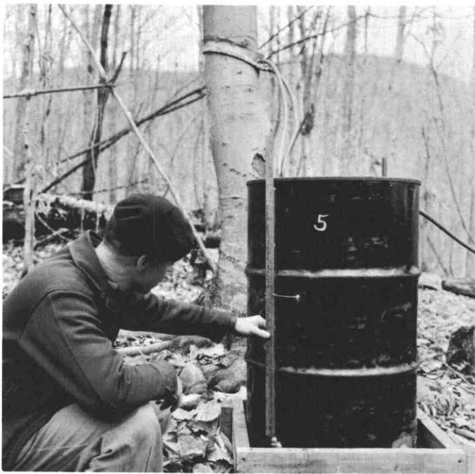
Figure 4. — Volumetric measurement of stemflow collected in 55-gallon drum. The rate of stemflow here necessitated use of two plastic drain tubes.
