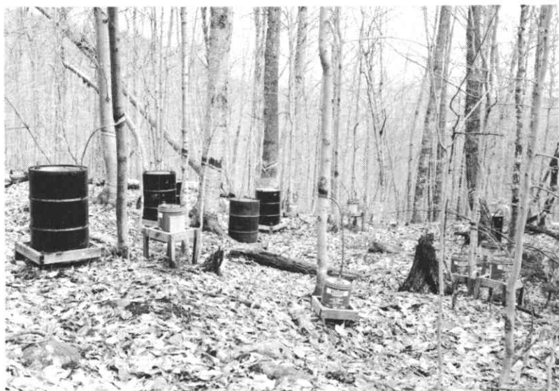
Figure 3. — The stemflow study area. Water running down tree stems was caught by metal collars and drained through plastic tubing to collecting drums and cans.
