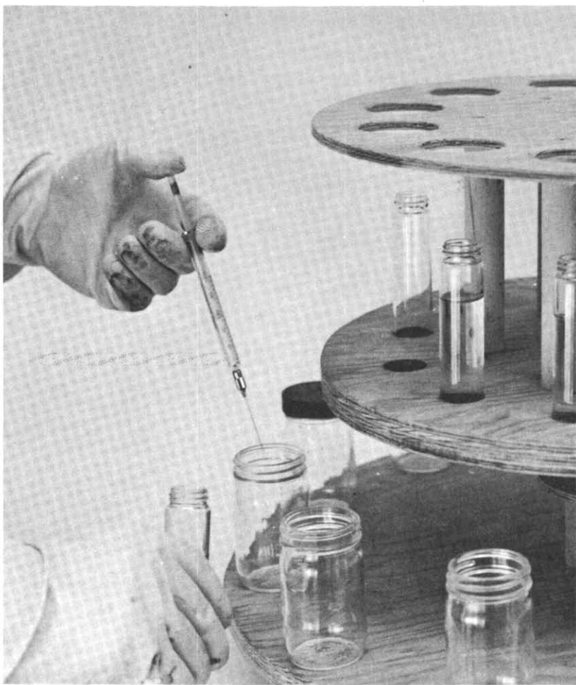
Figure 7. — An accurate syringe or micropipette is required for taking the 0.5-ml. sample for analysis.
