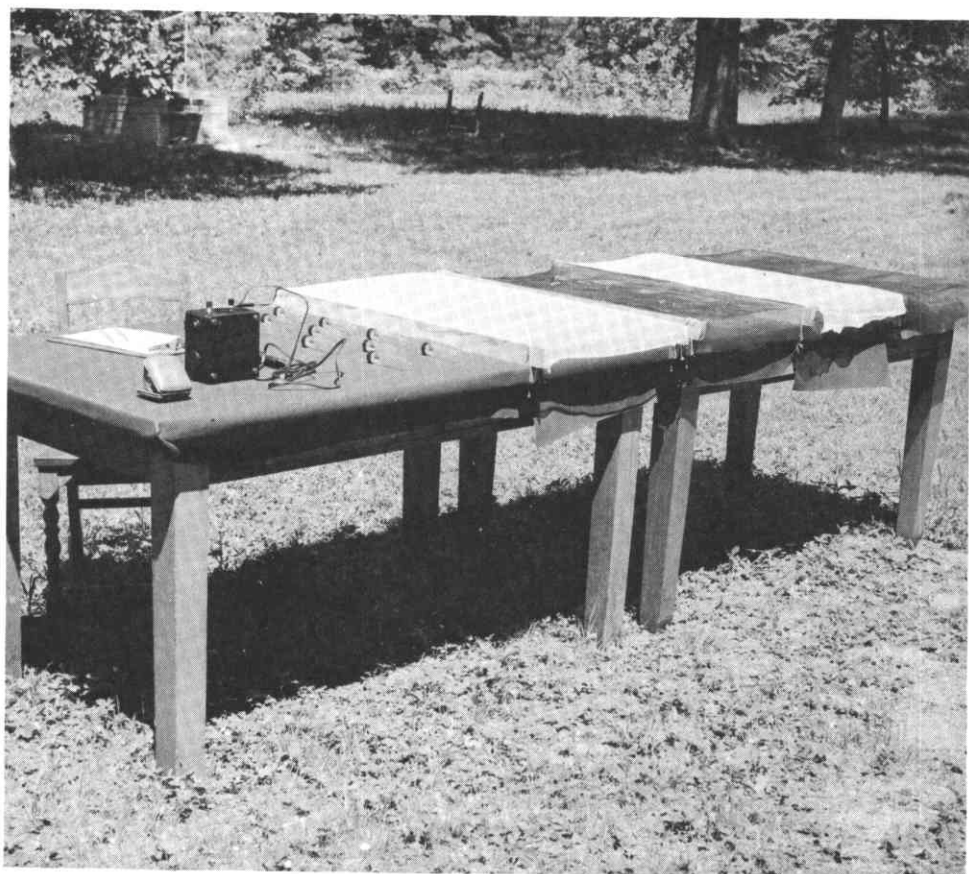
Figure 13.—Set-up for calibration. The four screens and open table top provide five different light intensities. The larger black instrument is the illumination meter, with target attached; the smaller is a clock for timing intervals between exposures.
