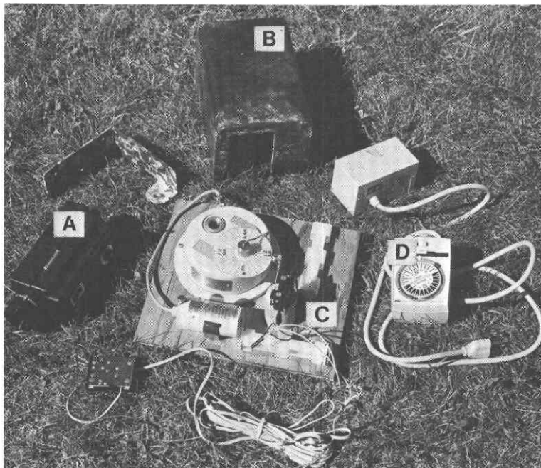
Figure 5.— The movie camera (A) is housed in a weather- and sound-proof box (B) and fixed in the required monitoring position. The system includes a battery-operated automatic timing device (C) which turns the camera off at night and on in the morning, or, when AC power is available, an AC-DC converter and automatic timing device (D) that serves the same function.
