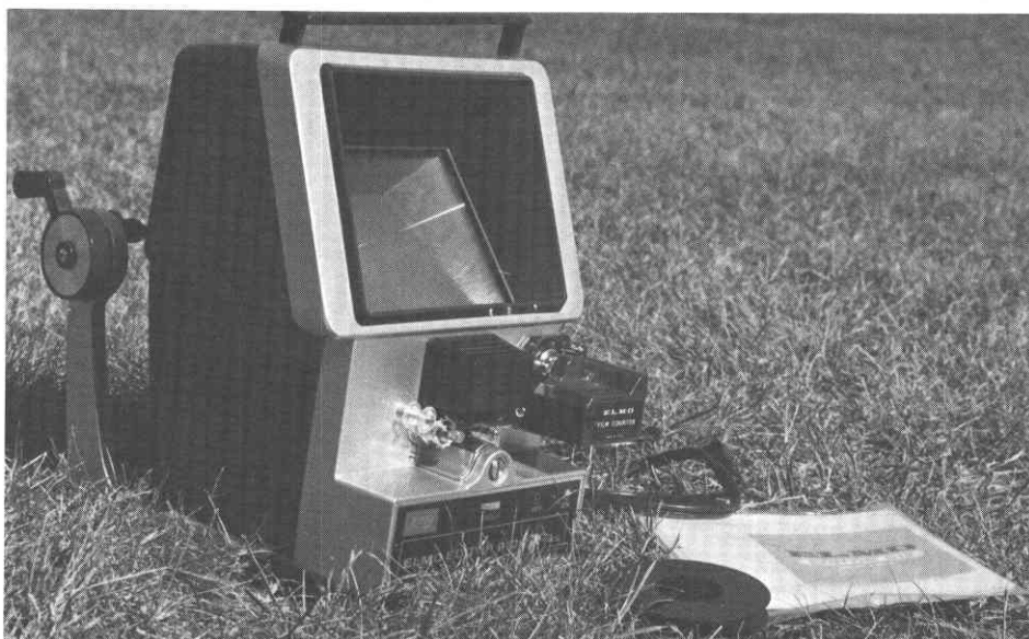
Figure 6.— Editing machine for 8-mm movie film is used to view and analyze film taken by the automatic monitoring camera.
