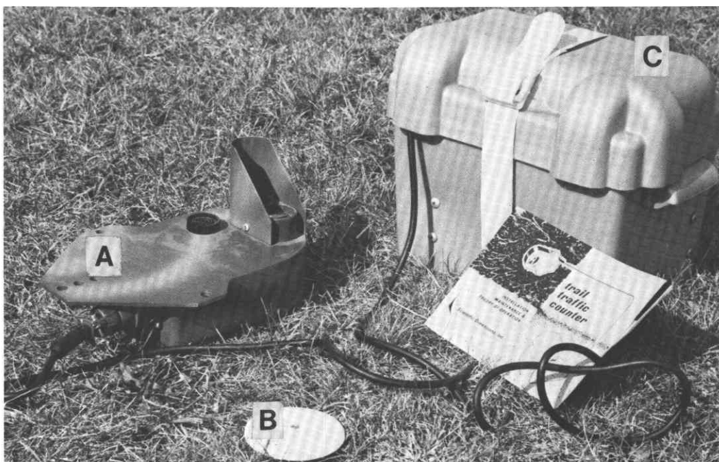
Figure 4.—The photoelectric counter (A) is inconspicuously mounted on a tree directly opposite a reflector (B), also affixed to a tree across the trail. The counter is wired to a battery in a box (C), buried nearby.
