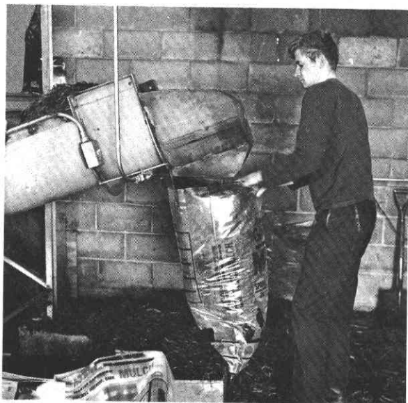
Figure 4.—Filling 3-cubic-foot open-mouth plastic bags with shredded hardwood bark mulch. Preset push-button limit switch is to the immediate left of the drop chute.
