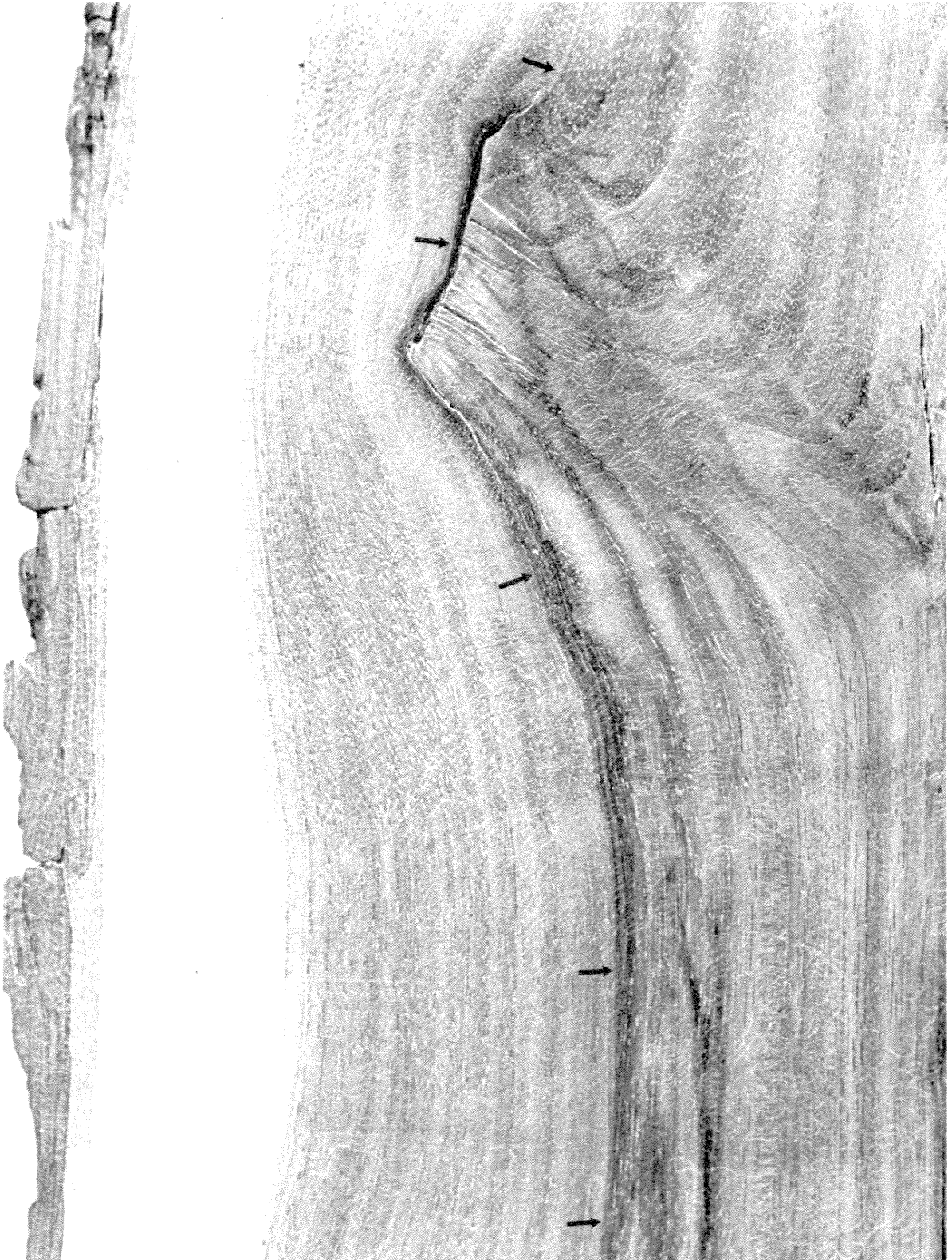
Figure 14.—Closeup of well-closed pruned stub in Tree 359. Note ring shake line at the barrier zone, and band of dark heartwood (arrows).
