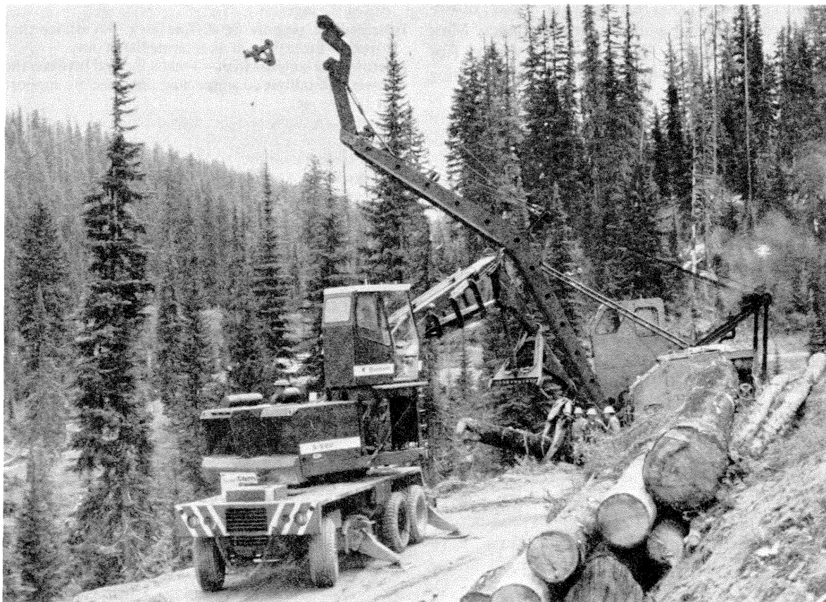
Figure 4.—A converted shovel at work in the western United States.
