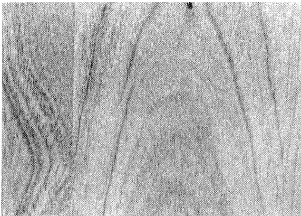
Figure 1.—Close-up of Serpentine end joint in cherry panel.
