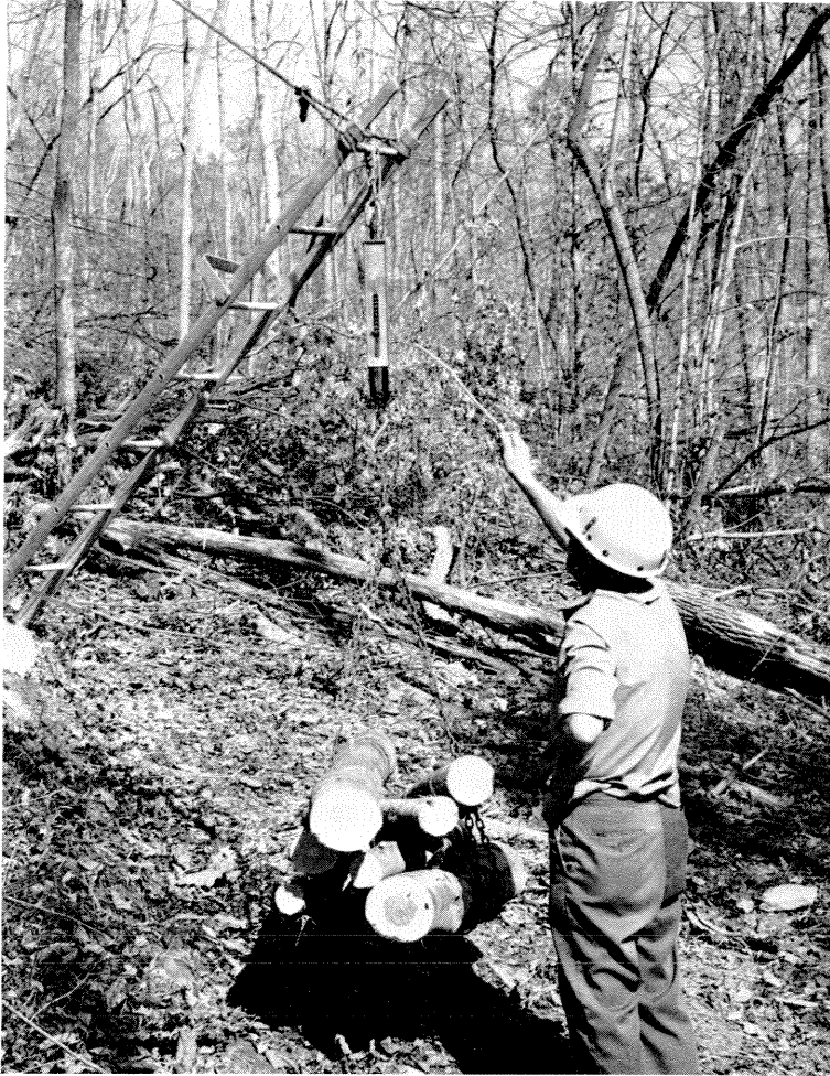
Figure 1. Weighing treetop residue in the woods with lightweight portable equipment.
