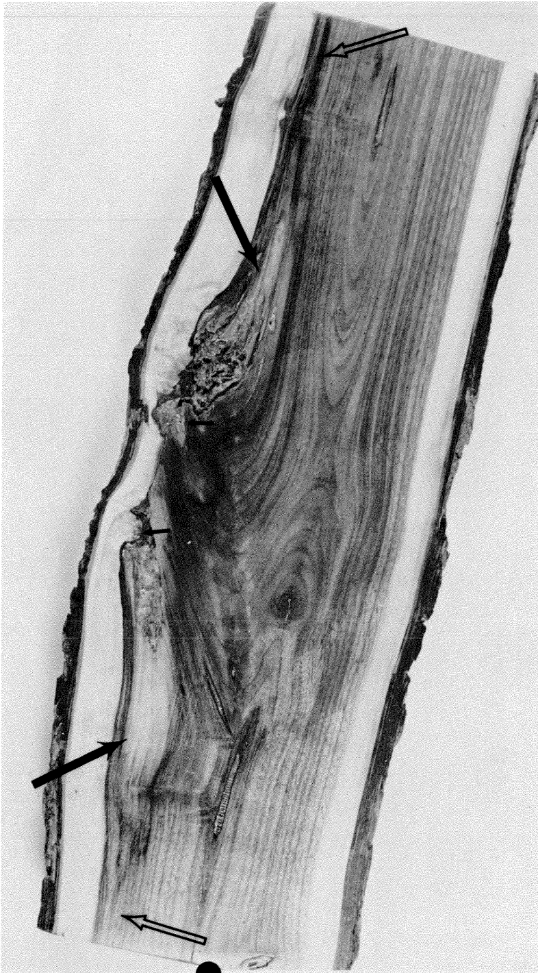
Figure 18.—Advanced decay (large arrows) associated with a flush cut dead branch on a very slow-growing tree. Note the position of the decay—it did not spread to the center of the tree as implied by the heartrot concept. The decay is advancing through discolored wood and is not spreading inward through nonaltered or nondiscolored heartwood. The
