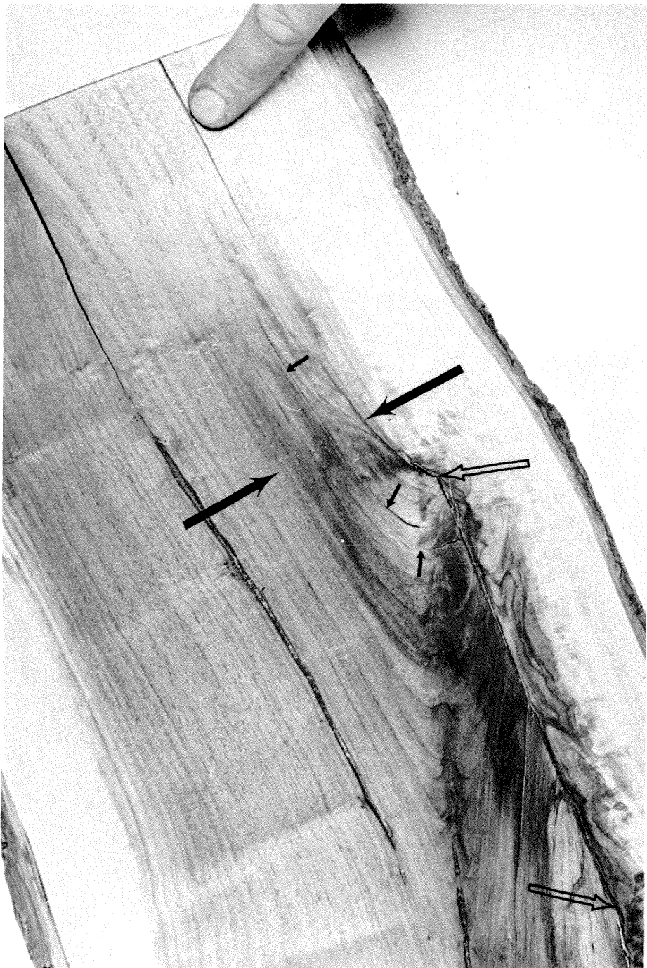
Figure 13.—A 7-inch, 13-year-old flush cut (open arrows). Note decayed wood beginning to form at the upper and lower limits. The large arrows show the dark band of discolored heartwood associated with the flush pruning wounds. The finger points to a large ring shake associated with the wound. The shakes usually opened more at the ends of the sample boards. The large open shake was
