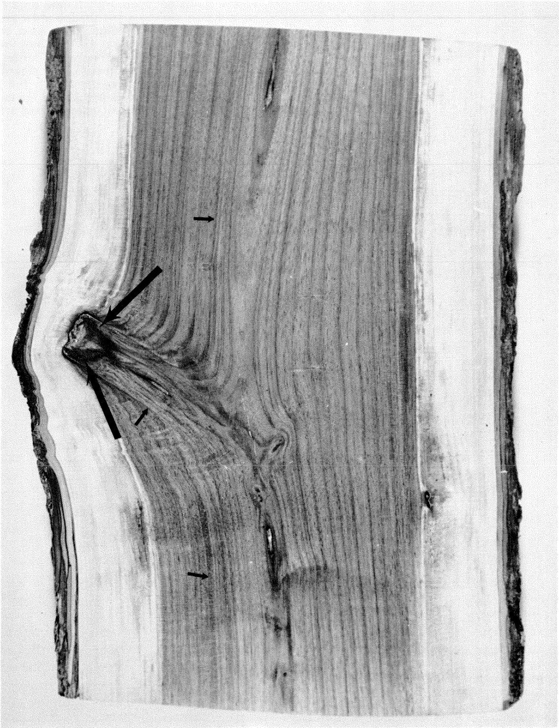
Figure 5.—A well-closed branch stub. When all systems function properly, the branch is enclosed in the stem. Even if some decayed wood develops, it will be confined by the branch stub chemical zone (large arrows). A slight bump may form as the stub wound is
