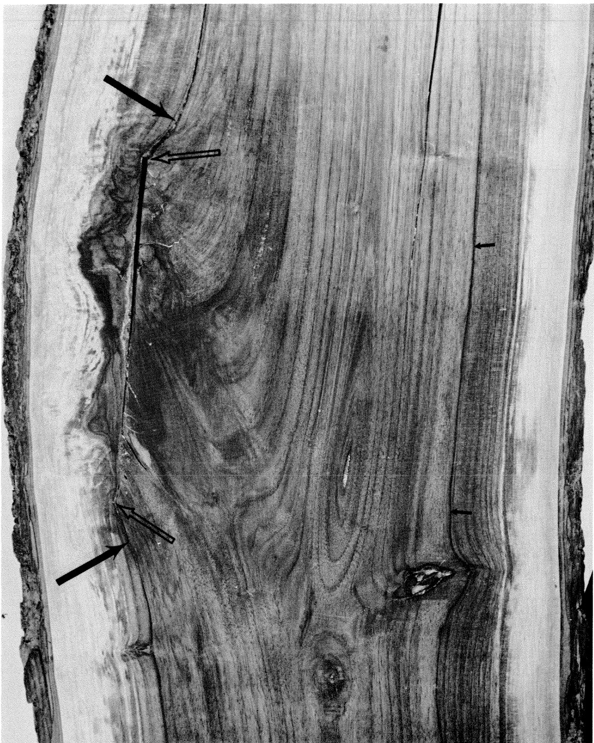
Figure 12. —A large flush cut similar to that shown in Figure 11, but 13 years later. The distance between the open arrows is 7 inches. The branch at the time of the cut was less than 2 inches in diameter. The large arrows show the large ring shakes that developed
