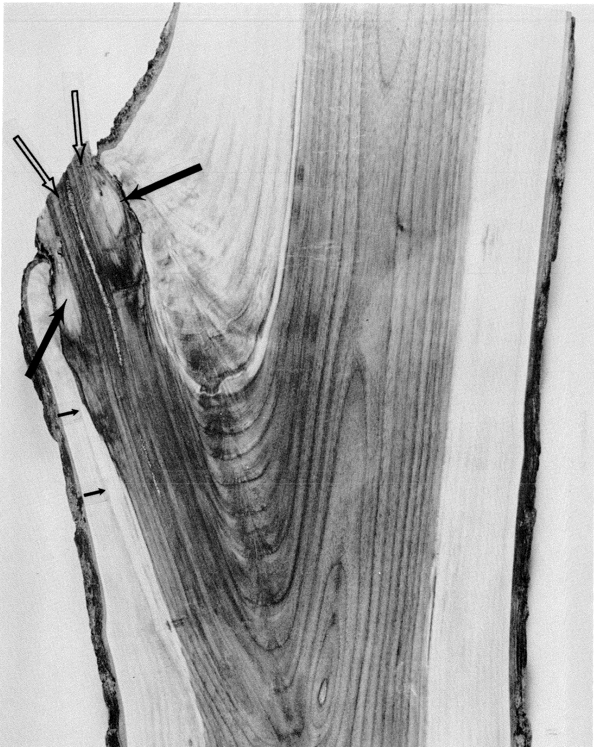
Figure 16.—Pockets of decay starting in discolored sapwood in a dead stub (large arrows). When decay develops in a stub it usually starts in the discolored sapwood and not the exposed heartwood, as is stated in the heartrot concept. Note that the heartwood in
