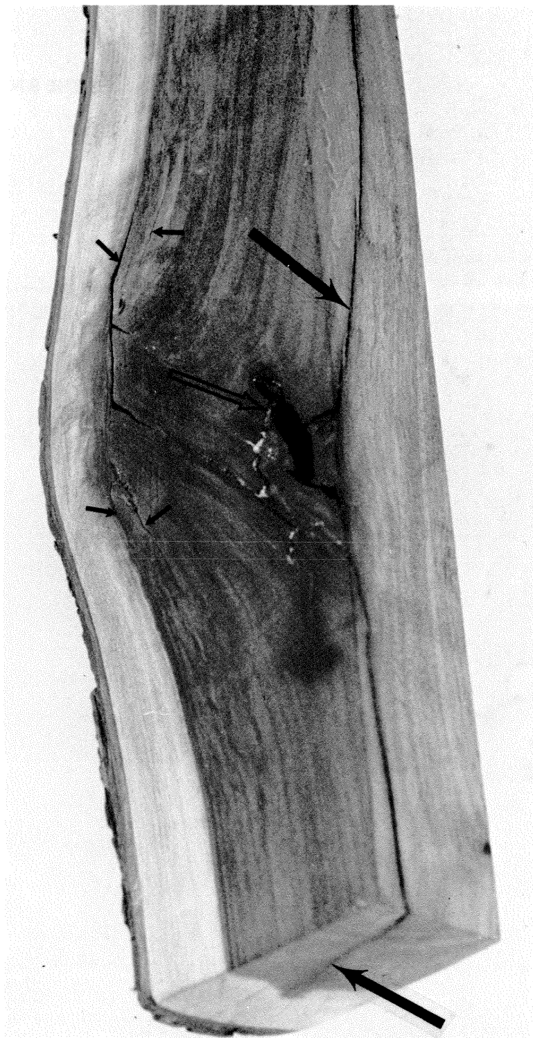
Figure 21. —A large radial seam was associated with this pruned stub (large arrow). Insects had infested deep into the stub (open arrow). Ring shakes were also present (small arrows). As wind or temperature extremes
