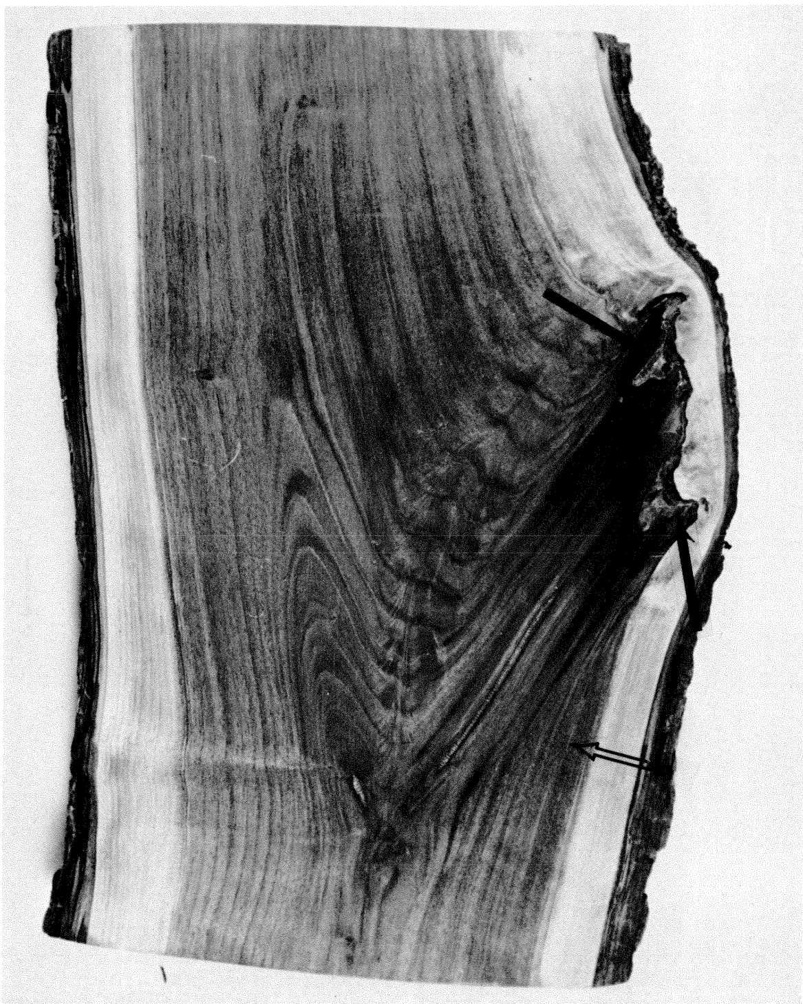
Figure 17.— Most of the time the tree's defense systems function properly, and even when decay develops in the discolored sapwood of the branch, it does not continue to spread into the tree after the branch falls. The large arrows show the old decay pockets
