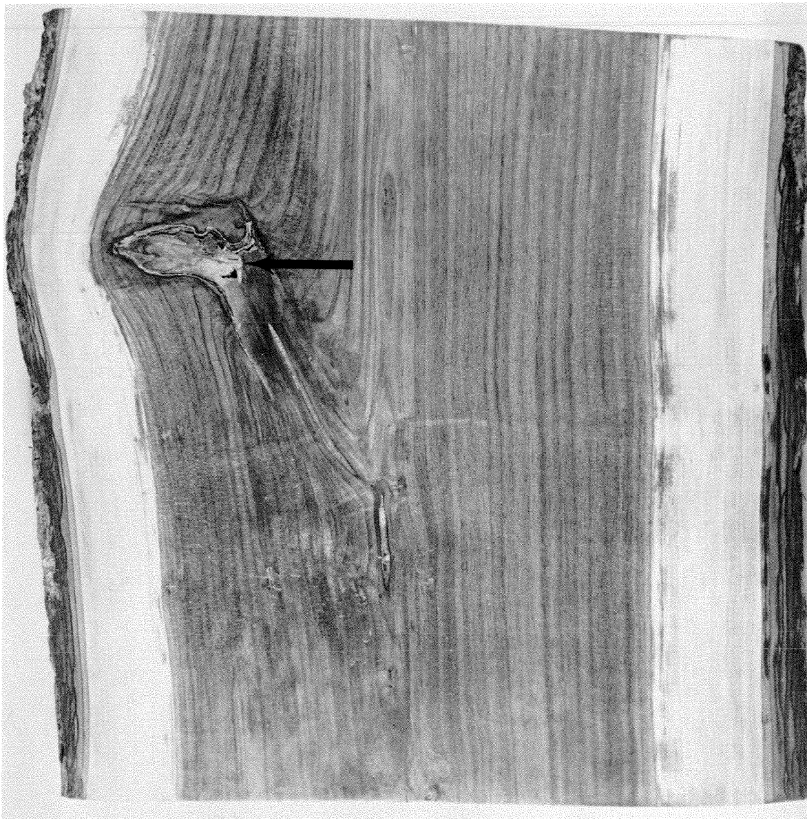
Figure 7.—An enclosed small stub. This stub broke before it fell from the tree, and the arrow shows the extent of the decayed wood and the cracked base of an old branch. The broken stub, even on this very small branch, greatly increased the time required for closure.
