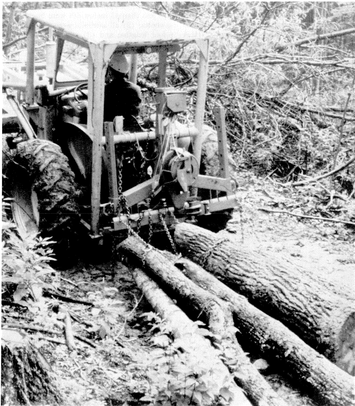
Figure 1.—Wheeled tractor with rear-mounted winch on standard three-point hitch used for skidding on Plot 1.
