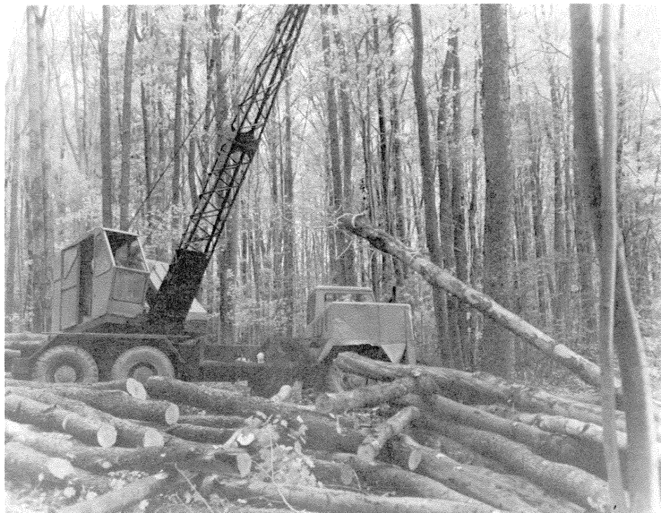
Figure 2.—Truck-mounted crane used to yard tree-length logs from thinned and clearcut blocks. Maximum yarding distance on slopes was 450 feet.
