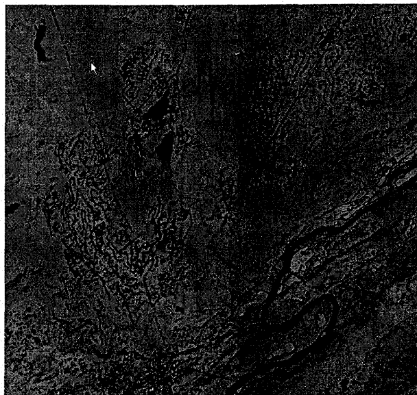
Figure 5. Land-cover map produced from the unsupervised classification of the first three principal components calculated from 5 bands: a SPOT 4 pan image and four texture images. Each of the four texture images was created using a 3x3 window and the algorithms: standard deviation, minimum, maximum, and average, respectively. Clusters of roads can be interpreted as suburban areas.
