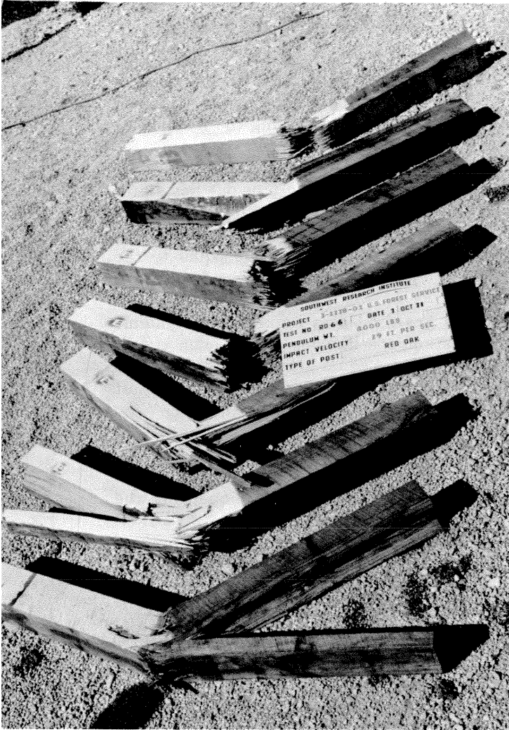
Figure 11.—Examples of wooden posts after impact testing.
