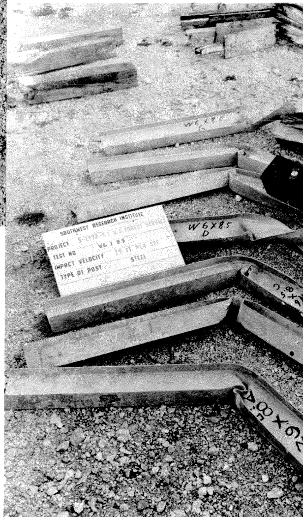
Figure 12.—Examples of steel posts after impact testing.
