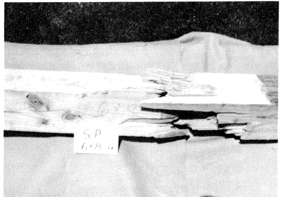
SP 68G. Three knots were located 4 to 6 inches above the clamp on the tension face. No knot disoriented the grain for more than one-third the width of the tension face. Post impact strength: above average for the SP 68 series.
