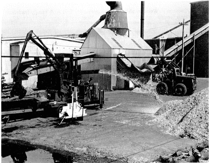
Figure 19.—Forty percent of Maine's primary manufacturing plant residues are used for fuel, mostly as industrial fuel. At this sawmill in Sanford, Maine, plant residues and roundwood chips are mixed to fuel boilers for steam and heat for kilns, and to provide heat and co-generated electricity to the mill. Excess electricity is supplied to the local electric company during non-peak hours ( Maine Forest Service ).
