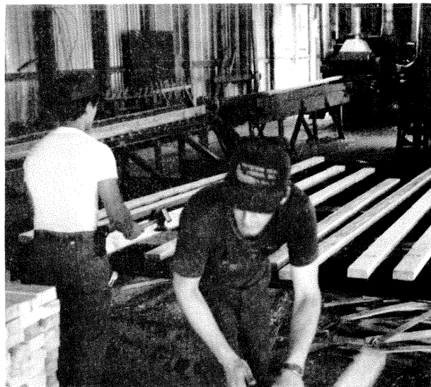
Figure 1.--Quality-assurance and consumer acceptance are foremost at this Vermont sawmill where spruce and fir lumber is planed, graded, grade-stamped, and sorted by grade. (Vermont Department of Forests, Parks and Recreation).
