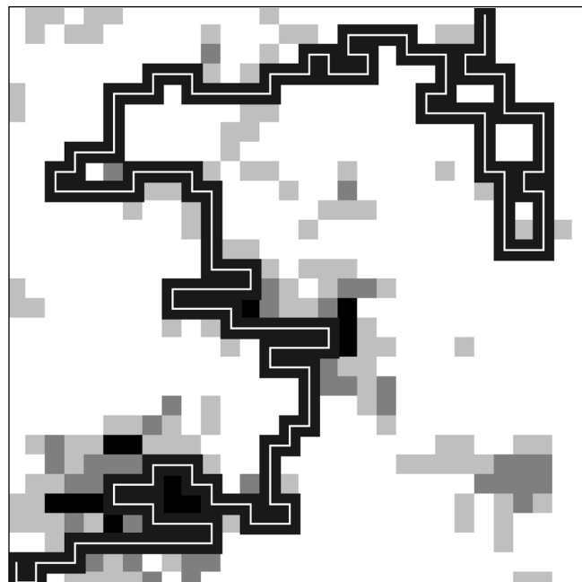
Figure 4.—Example of a selected survey strip with unrestricted guided transect sampling, with which the first stage strips are skipped and transects are simulated directly through the whole area of interest.
