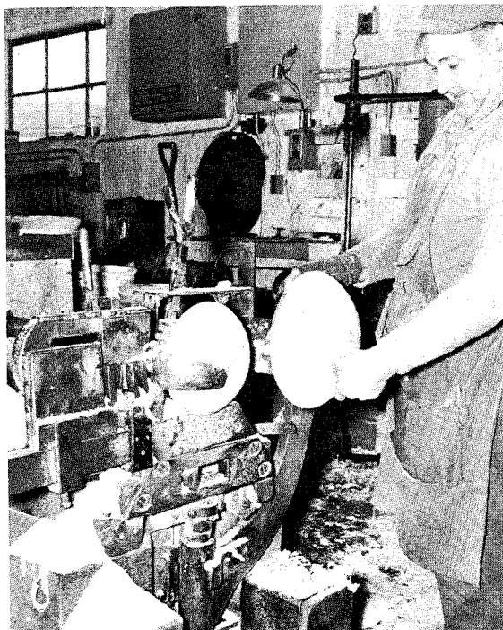
Figure 6.—Vermont's only remaining wooden bowl mill, at Granville, uses a specially designed lathe to cut bowls from hardwood bolts.
