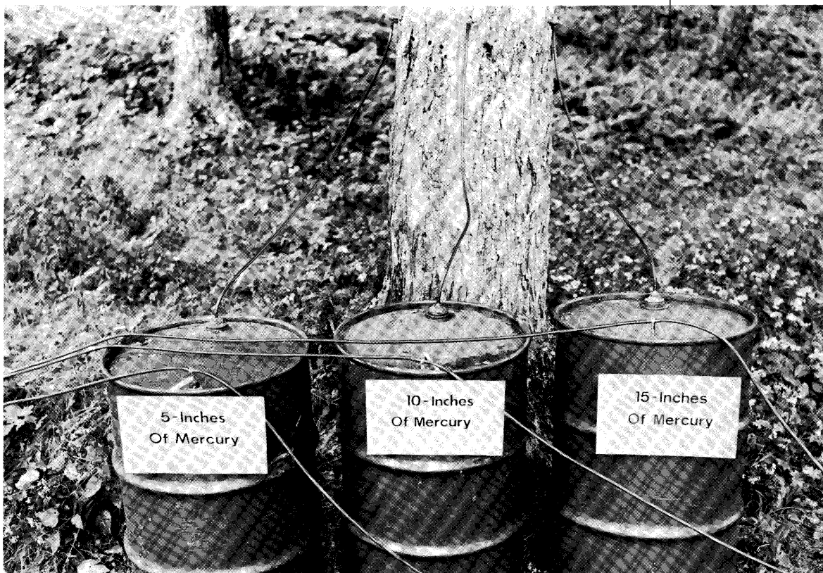
Figure 1.—Sap from each taphole was collected in individually sealed 55-gallon steel drums.
