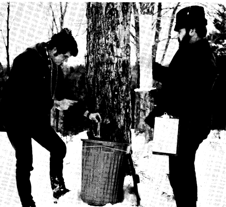
Figure 1.—Left, sap-flow rate was measured with a stopwatch and graduated cylinder. Right, sap volume was measured to the nearest \frac{1}{2} liter.
