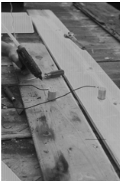
Figure 1a. — Surface-mounted sensor for AE termite detection device. Boards in the background are 3- by 20-cm (1- by 8-in.) ponderosa pine.
