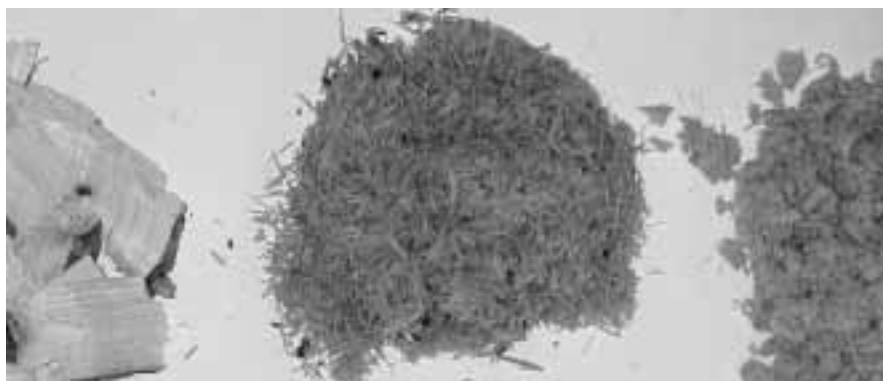
Figure 2. — Tornado pin-chips (center) have high length-to-diameter ratio fiber bundles (0.5- to 1.0-mm diameter by 10- to 15-mm length) with a minimum amount of fines. Conventional chips (left) and refined pulp fibers (right) are for reference.
