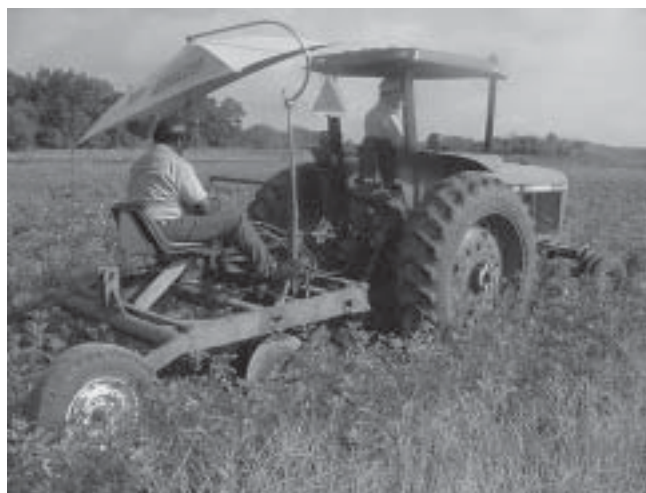
Figure 3 —Rolling coulter blades used to manage lateral roots in bareroot seedling beds.
