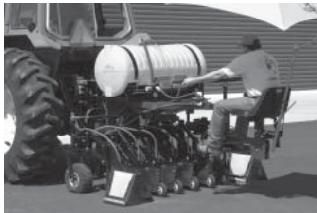
Figure 3 —MTDC's improved shielded herbicide sprayer is being evaluated in Virginia.
