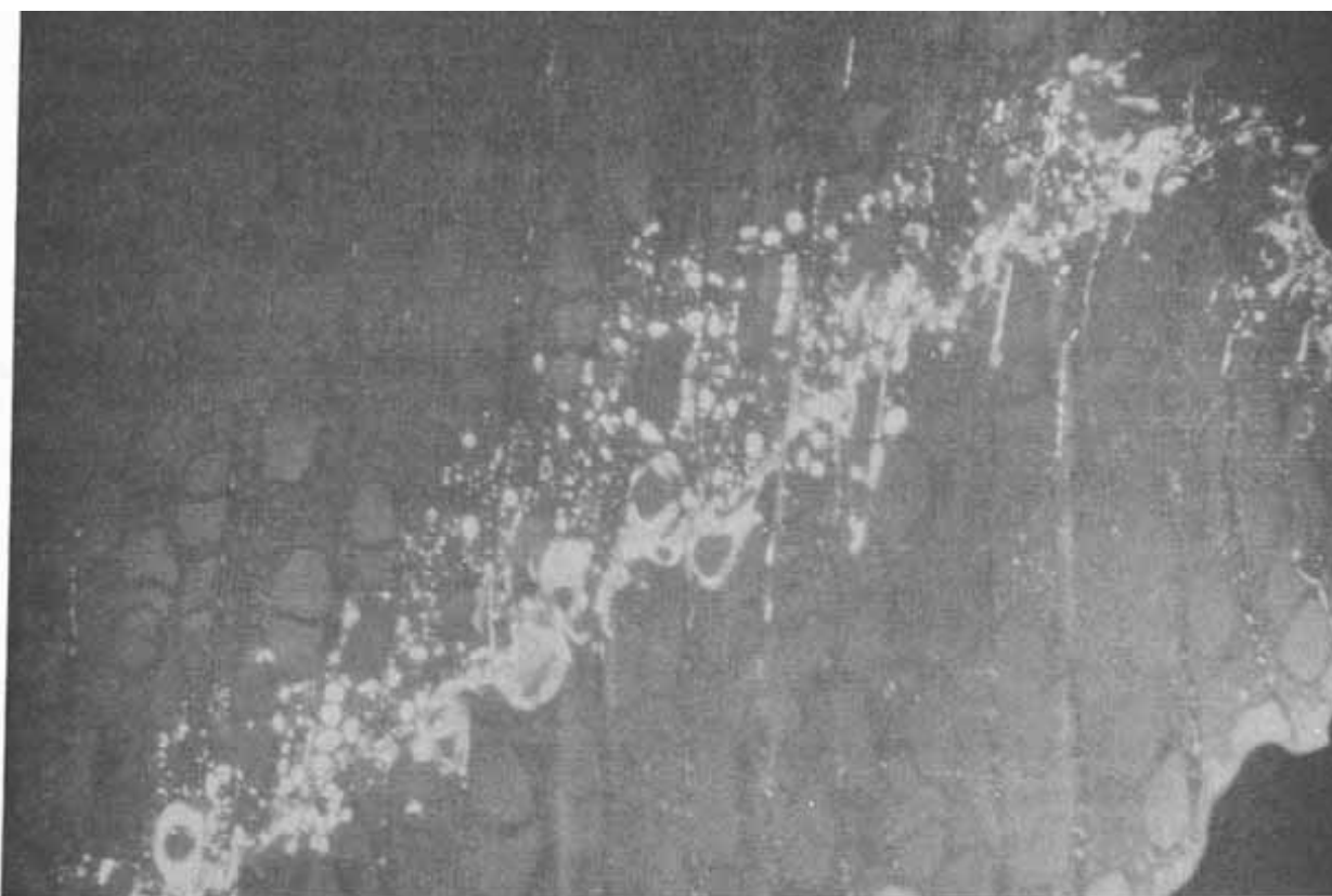
Figure 19.-- Resin penetration: photomicrograph under fluorescent light for isocyanate-bonded aspen flakes
