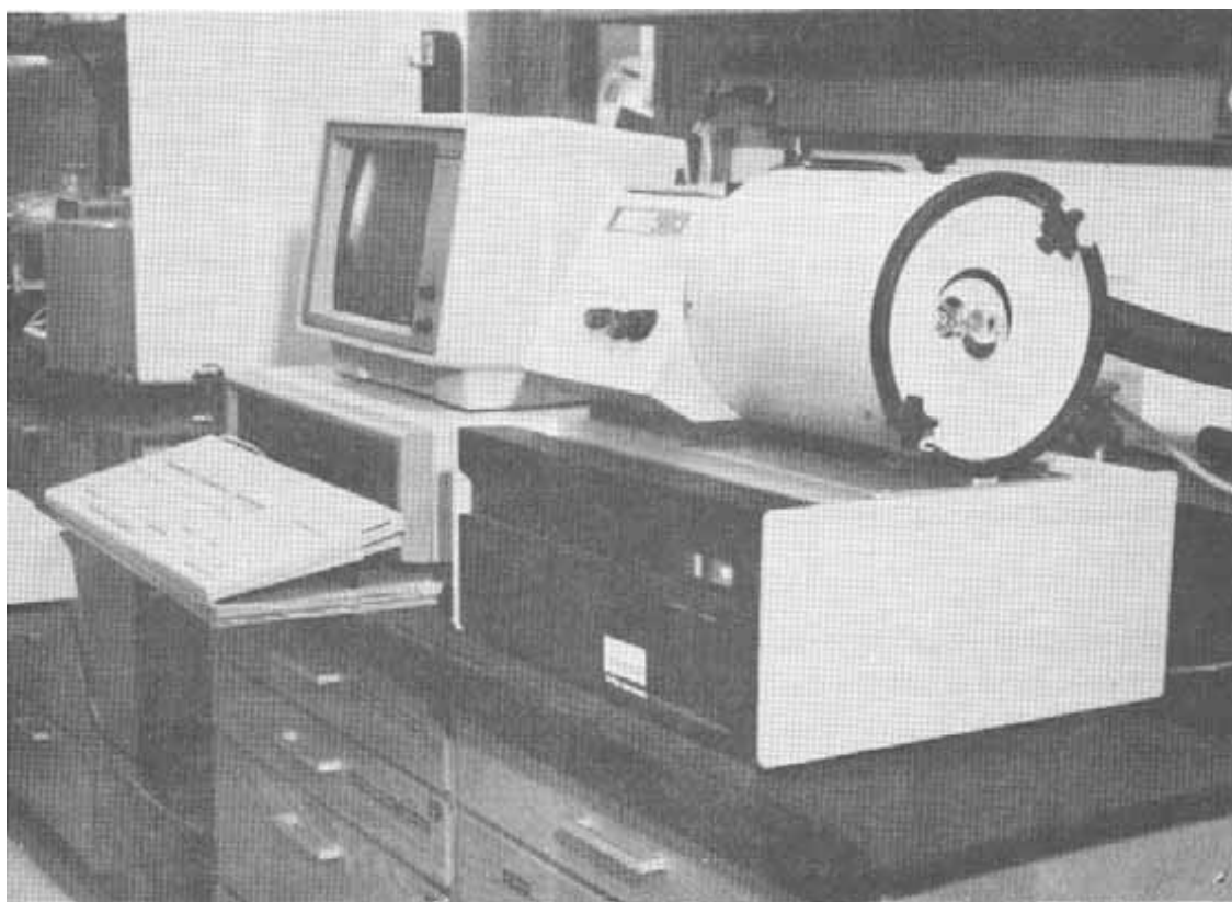
Figure 1.- Du Pont 983 dynamic mechanical analyzer
