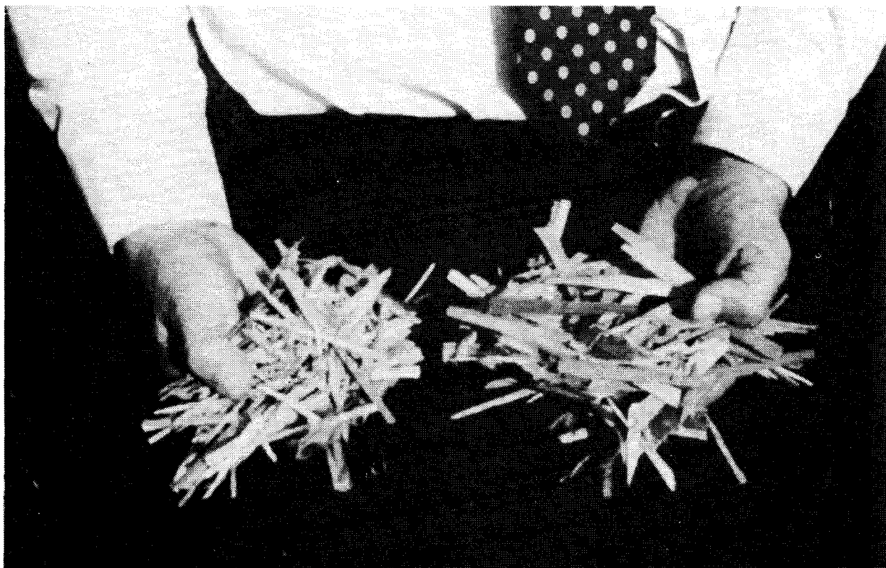
Figure 1. --Flakes used for large-scale panel fabrication; left side is red oak flakes, right side is sweet gum flakes
