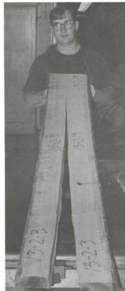
Figure 7.—Severe growth stresses produced this split, which lengthened during drying. (M 147 632)
